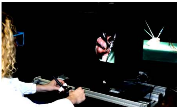
Fig. 1 Master console with haptic input devices, stereoscopic screen, and slave system in the background
